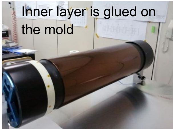
Cathode is rolled on the mold and glued in a vacuum bag
