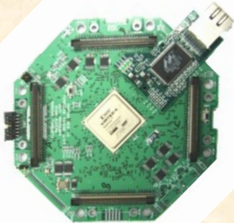
Node processing board
