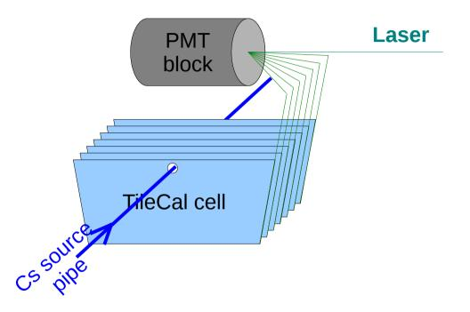
• Cs 137 -source transported by hydraulic system through every scintillator composing TileCal cells.
