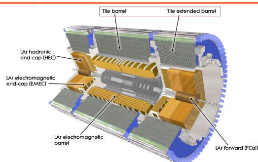
Sampling calorimeter (plastic scintillator/iron)
