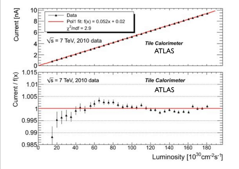
An average anode current for A13 cell of the TileCal is shown as a function of the instant luminosity on full data sample taken in 2010. The errors on the current are the quadratic sum of the statistical and systematic errors. The red lines are obtained from the linear fit of the data points.
