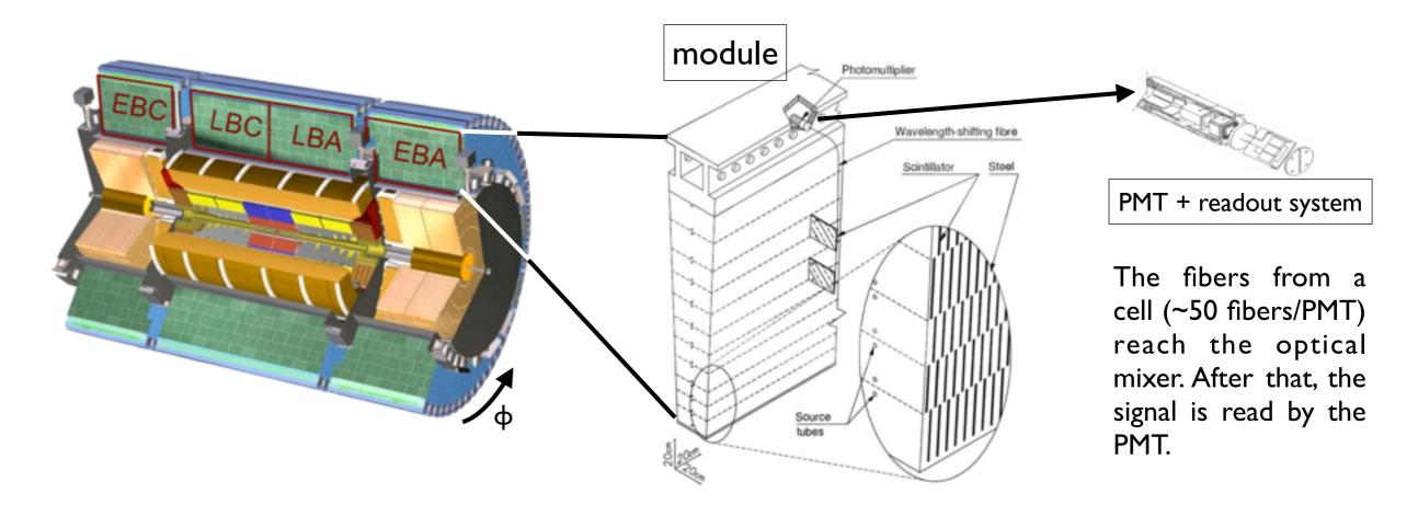
The readout architecture divides the detector in **four partitions**, there are two Long Barrels (LB) and two External Barrels (EB). Dividing the detector perpendicular through the interaction point we have the A and C sides.
