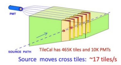
A Cs radioactive  $\gamma$ -source is moved through each scintillator tile by a hydraulic system.
