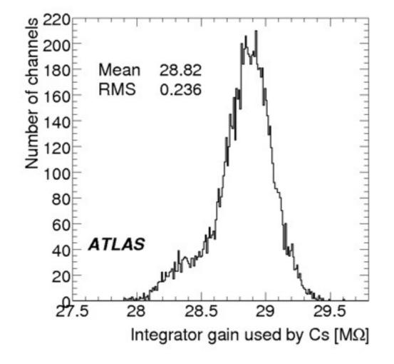
The gain variation is about 1%. The left tail is produced because 16% of the ADC cards come from different production batch.
