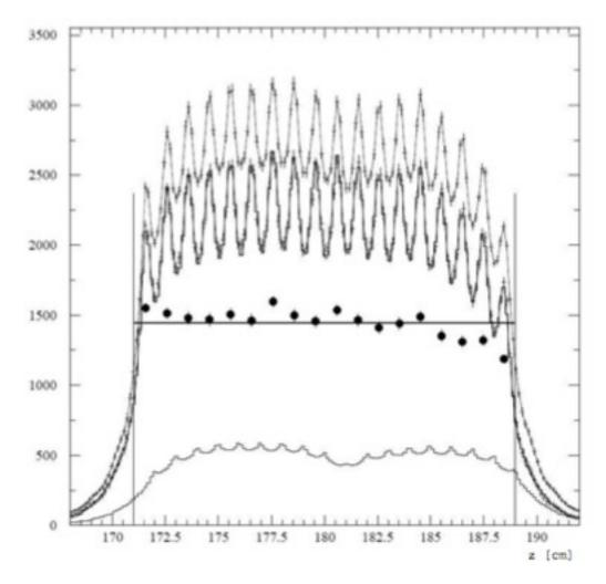
The Cs-source signal measured in one PMT as a function of the source position. The signal (middle curve) is obtained by subtracting the estimate leakage (bottom curve) from raw data (top curve). The individual tile amplitudes (full circles) are obtained by fitting the signal by a sum of pulse shape functions for individual tiles.
