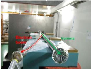
• Calorimeter-type Csl(Tl) scintillator + PMTs
