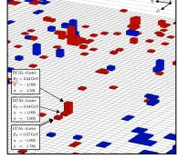
Calorimeter deposits before and after removing muon deposits
