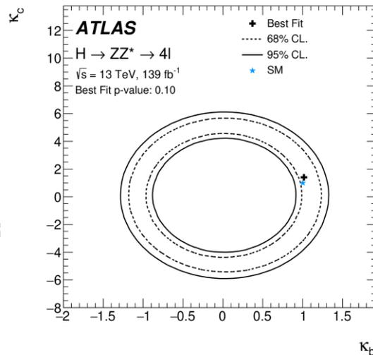
Observed direct constraint on the charm Yukawa coupling modifier  $|\kappa_c| < 8.5$
