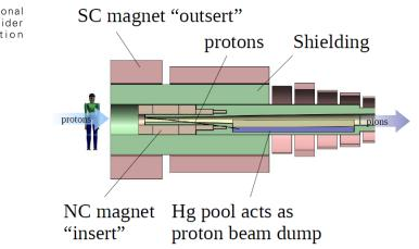
Hybrid design (superconducting + conventionnal magnets)
