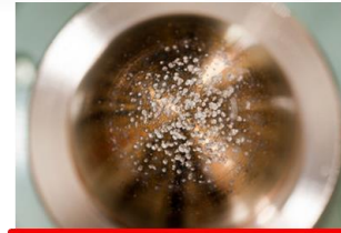
Damage on a 805 MHz rf cavity immersed in a multi-T magnetic field.
