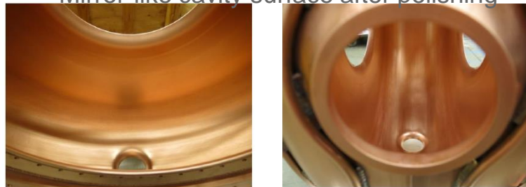
Mirror-like cavity surface after polishing
