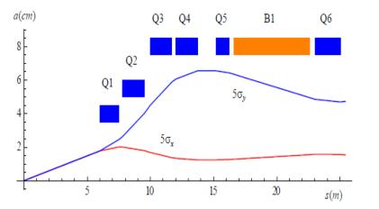
Beam sizes and aperture of the FF magnets  $a \ge 5\sigma_{max} + 1 \text{ cm}$ , B=8T in dipole. L<sub>B</sub> = 1.5 to 1.7 m in quads and 6 m in B1 Cross-sections and good-field regions ( $|\delta B/B| < 10^{-4}$ ) of Q1, Q2 and Q3-Q5 quads with G = 250, 187 and -130 T/m, respectively
