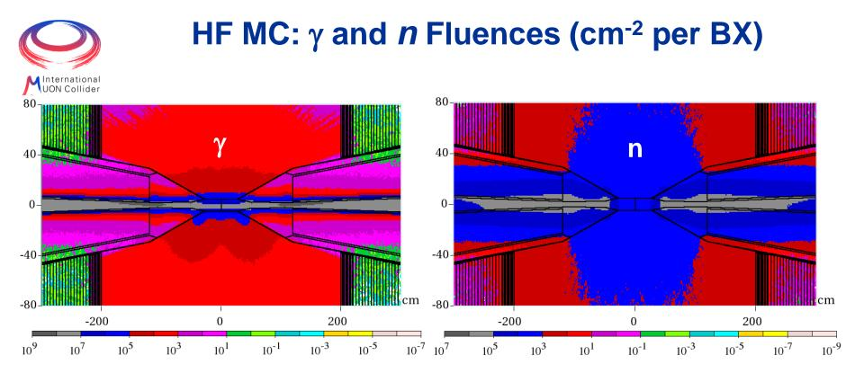
In central detector, the photon fluence is noticeably larger than in the LHC detectors while for neutrons it is much lower
