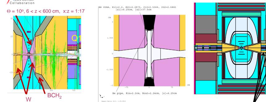
**Optional source term scoring at Black Hole:** the outer surface Of the Be pipe and nozzle as well as the IP side of the SS surface Nikolai Mokhov, Fermilab, May 20, 2021 Sophisticated shielding (**SS**): W, iron, concrete & BCH<sub>2</sub>
