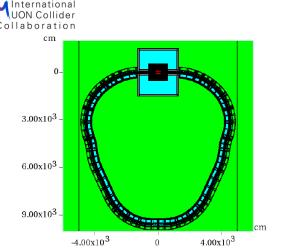
HF Muon Collider with IR, MDI and SIDlike detector with SVD and tracker model based on that of the CMS detector upgrade. The circumference is about 300 m. Simplified tunnel and detector hall geometry.
