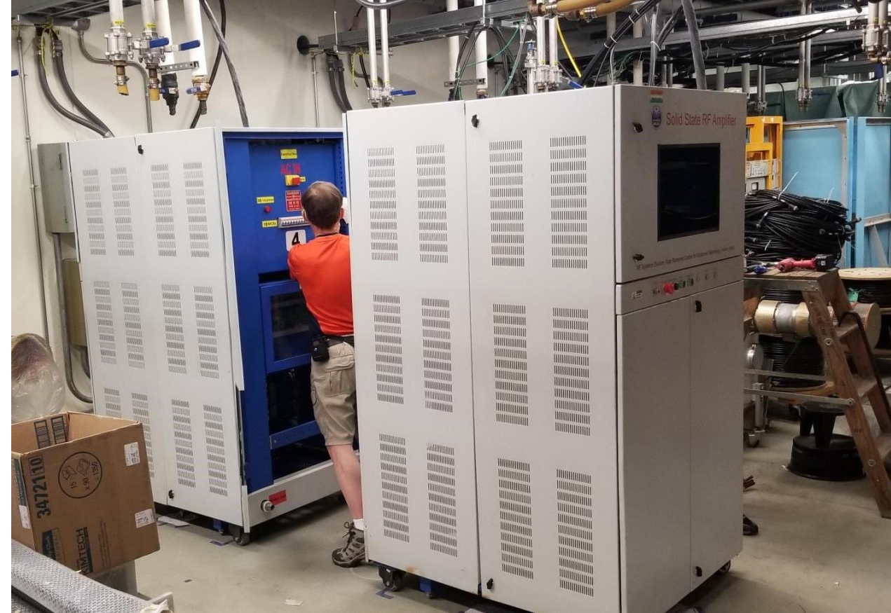
RRCAT 40 kW 650 MHz prototype being assembled, in preparation for testing
