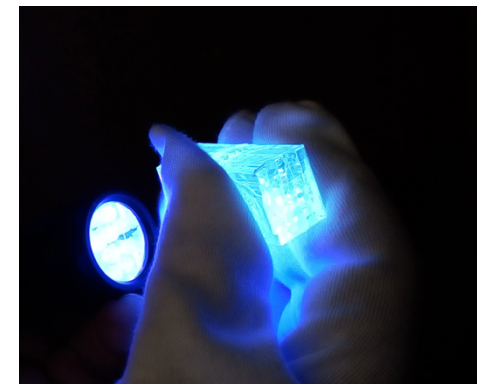
first prototype detecting module made of rectangular fibres.
