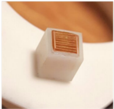
CdSe/CdS core crown nanoplatelets (CC NPLs) drop-casted film Effective deposited mass equivalent to 20 \mu m
