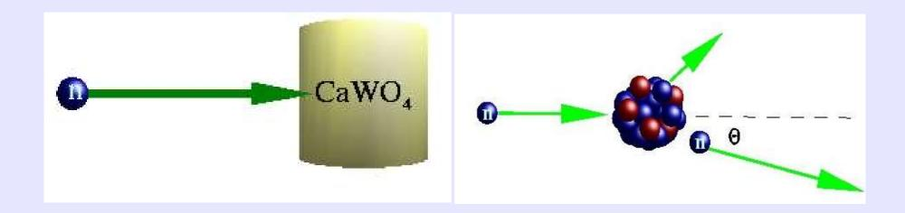
Target: small cylinder of CaWO4 (4cm height, 4cm diameter)
