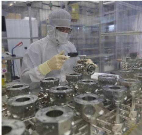
Precise mounting of feedthrough on body in clean room Photo: D. Nölle
