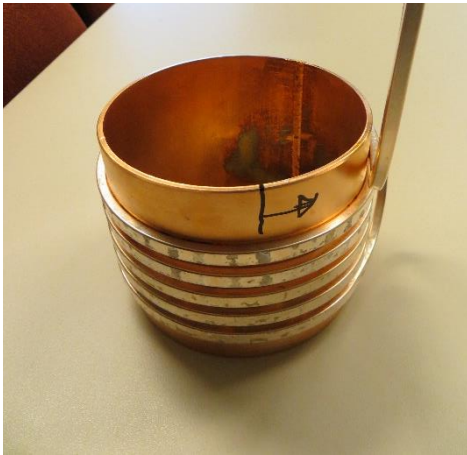
Brazed coil and UT-image of contact surface between coil and tube
