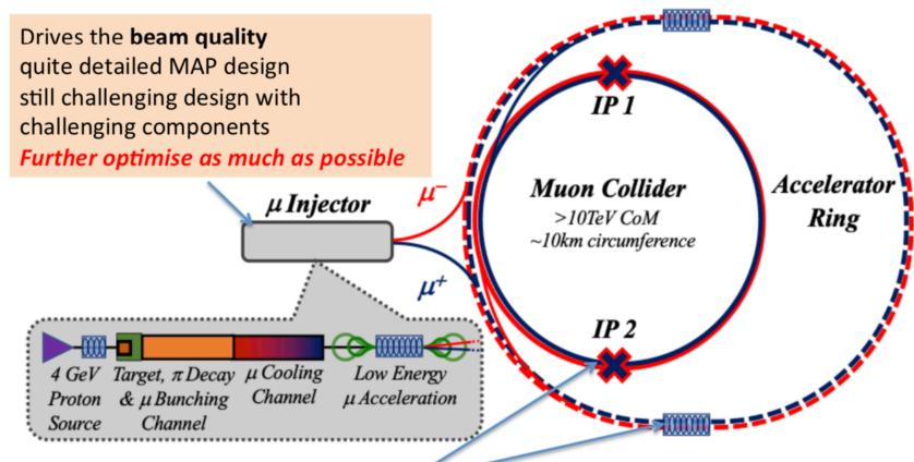
**Cost** and **power** consumption drivers, limit energy reach e.g. 30 km accelerator for 10/14 TeV, 10/14 km collider ring Also impacts **beam quality** Drives **neutrino radiation** and **beam induced background** *Improve compared to MAP design and design for high-energy*
