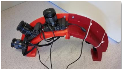
HD camera system for tunnel dome view
