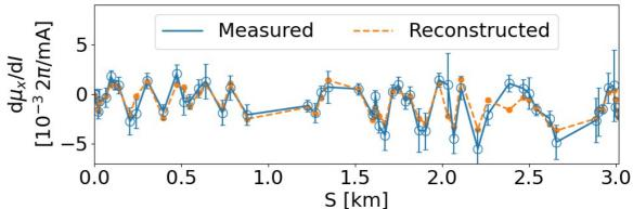
Using 20 negative kickers and the rest slightly positive Result in large kicker strengths Result changes with different max constraint
