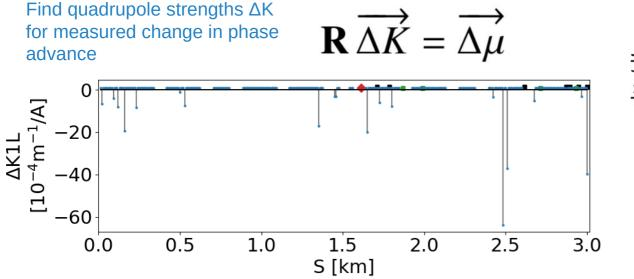
Red diamond: injection kicker Black: horizontal collimator, green: vertical collimator Constraints: K1L<sub>max</sub> = 2e-4
