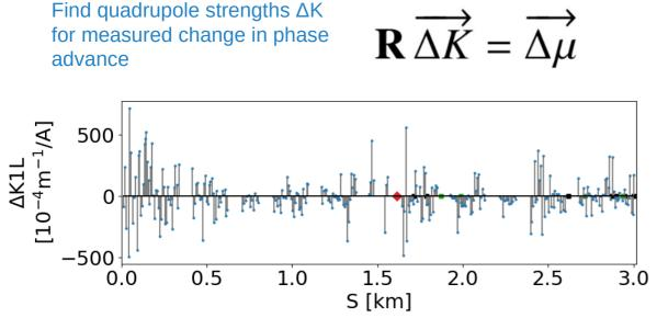
Red diamond: injection kicker Black: horizontal collimator, green: vertical collimator
