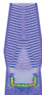
Simulated tomographic reconstruction after 1 h exposure time assuming a full detector coverage of the blast furnace
