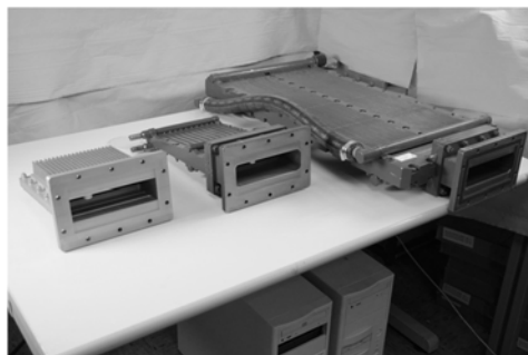
Three WR650 ferrite loads, 200W air cooled, 500kW water cooled and 5MW water cooled (from left to right)
