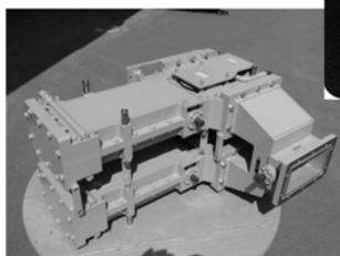
WR650 1MW isolator made of two 3-port circulators, two E-tees and two ferrite loads
