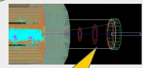
Forward Detector for Phase-2 for tagging <sup>3</sup>He<sup>++</sup> ions
