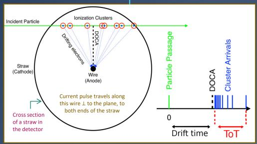
• So from simulations, numerically compute the path length (dx) from ToT and then get a measure of specific ionization (dE/dx) of each incident particle as edep  $\div$  dx.
