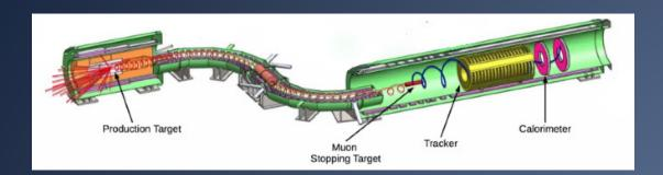
Mu2e will search for Charged Lepton Flavor Violation, using a cylindrical straw tracker for detecting particles.
