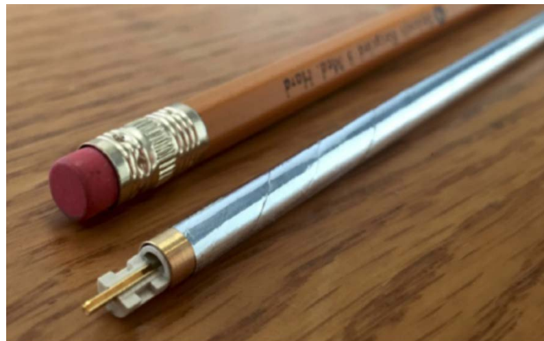
Straw tube (with termination) compared to a pencil
