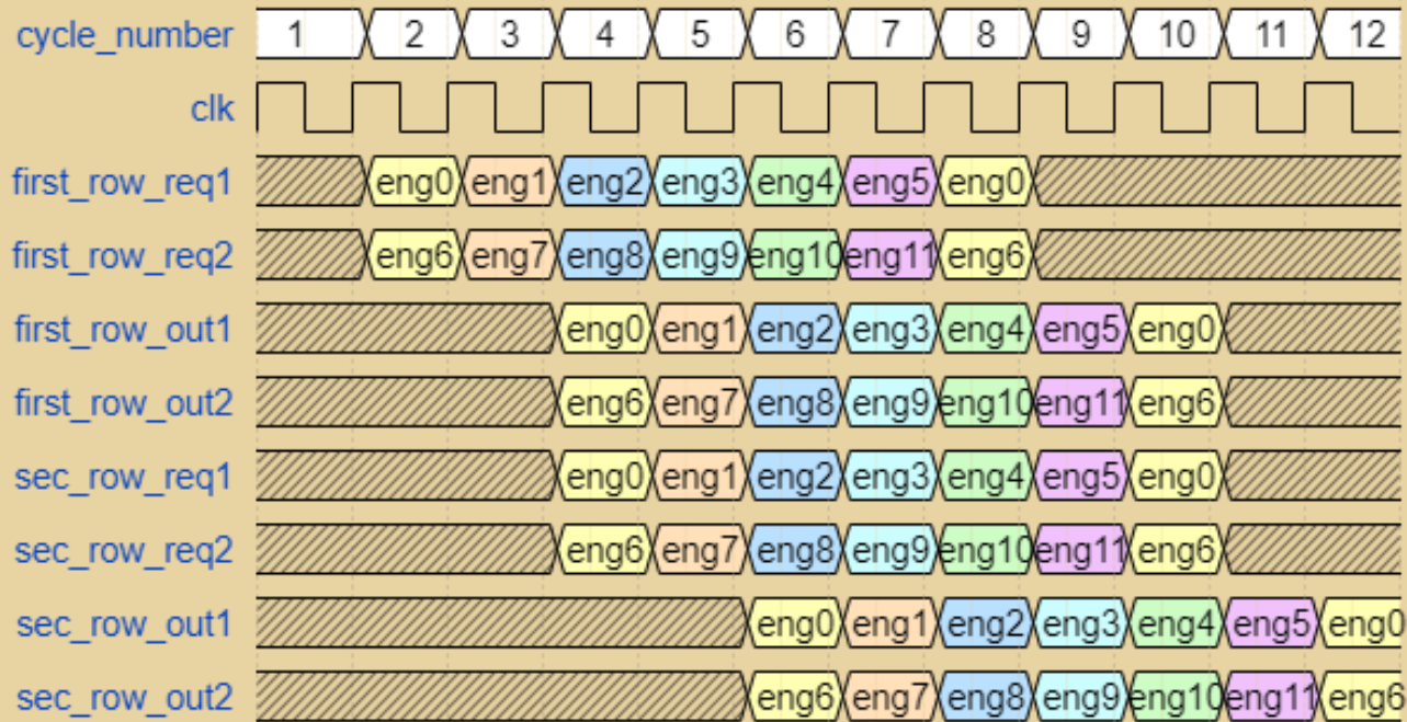
Figure 12: Timing diagram for the engine offsets for accessing centralized ROM system.
