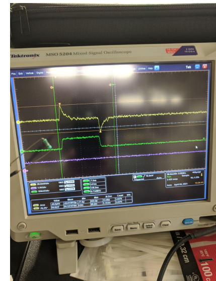
Injected charge seen on a scope
