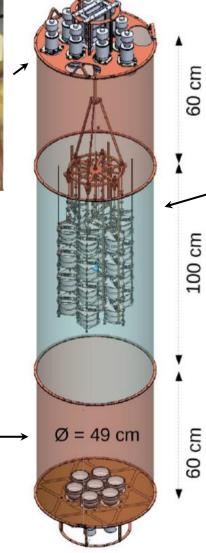
810 wavelength shifting fibers coupled to 90 SiPMs
