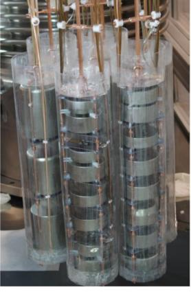
New TPB coated nylon minishrouds to reduce attraction of <sup>42</sup>K ions (from decays of <sup>42</sup>Ar) to n<sup>+</sup> surface
