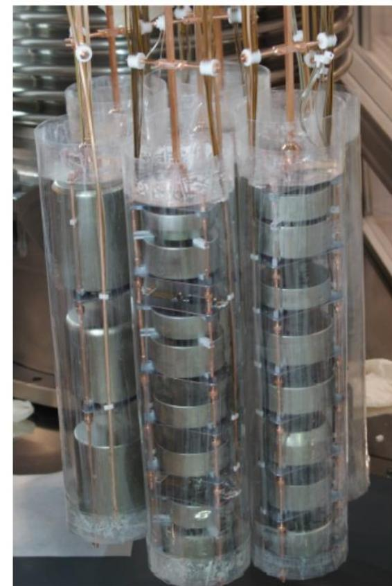
New TPB coated nylon mini-shrouds to reduce attraction of
