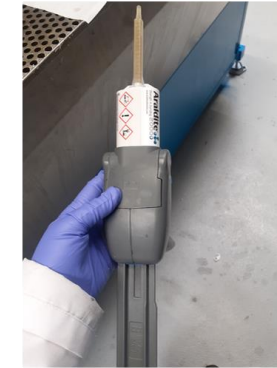
After cleaning the surface with acetone, used Araldite 2011 , spread a little amount through spatula
