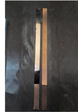
Cut in the proper dimensions, and put Teflon tape on one side and also on the unbonded ends(that will be clamped in the grips)
