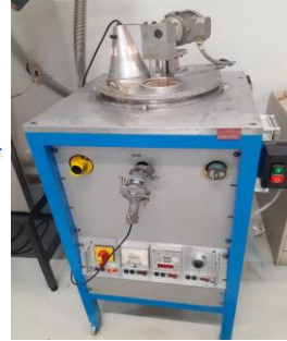
Vacuum degassing till all bubbles are gone
