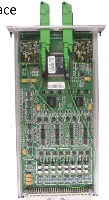
LHC acquisition module (BLECF)
