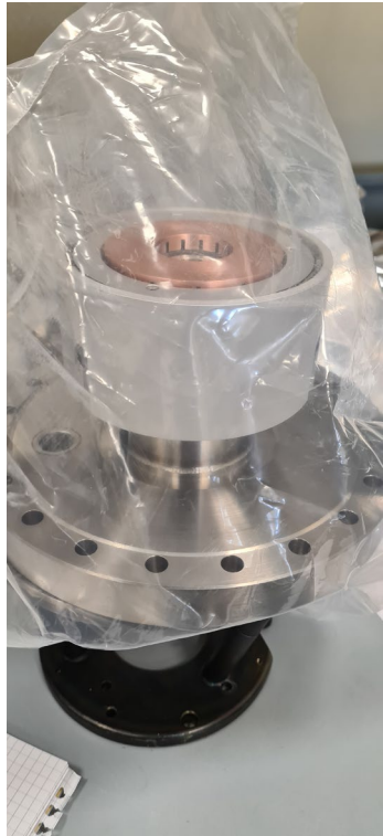
Commercial 4 " magnetron source
