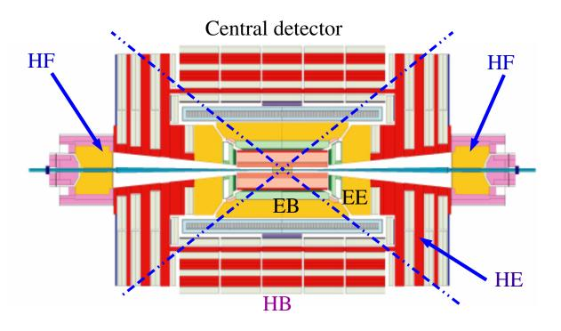
Electromagnetic Barrel Calorimeter (EB):  $|\eta| < 1.5$ Electromagnetic Endcap Calorimeter (EB):  $1.5 < |\eta| < 3.0$ Hadron Barrel Calorimeter (HB):  $|\eta| < 1.3$ Hadron Endcap Calorimeter (HE):  $1.3 < |\eta| < 3.0$ Hadron Forward Calorimeter (HF):  $3.0 < |\eta| < 5.2$ CMS offers perfect rapidity coverage to measure jets
