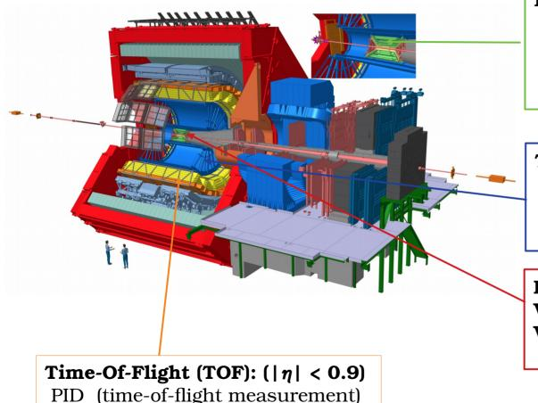
Inner Tracking System (ITS): ( $|\eta| < 0.9$ ) 6 layers of silicon detectors Tracking, vertex, Particle identification (PID)
