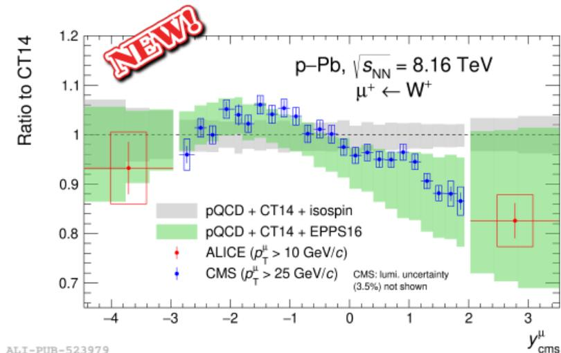
ALICE results in agreement with the trend at the edges of the CMS acceptance. Shows the relevance of providing measurements at large rapidities for nPDF determination.
