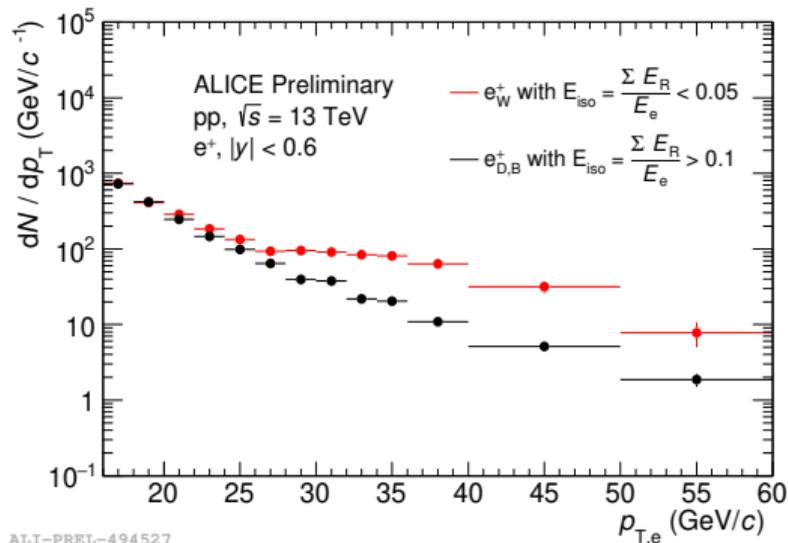
Background contamination evaluated from MC- and data-based methods and subtracted.
