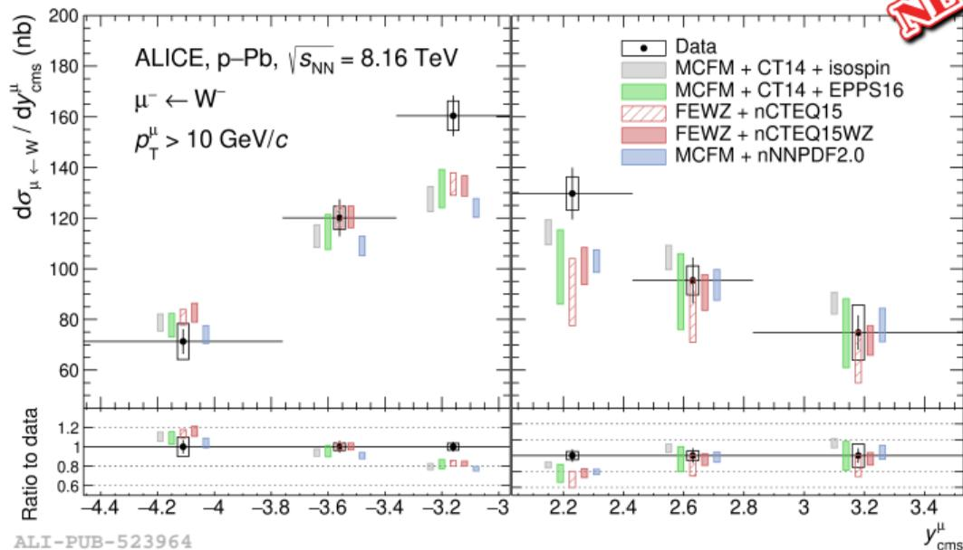
⇒ ability to constrain the slope of the evolution of the nPDF vs. rapidity (i.e. vs. Bjorken- $x$ ).
