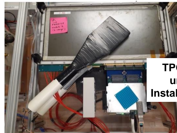
TPC GEM & support assembly complete!
