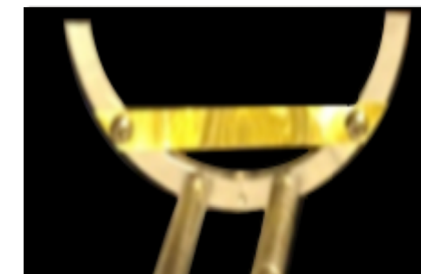
Au-Target = 0.25mm thickness 1% interaction probability
