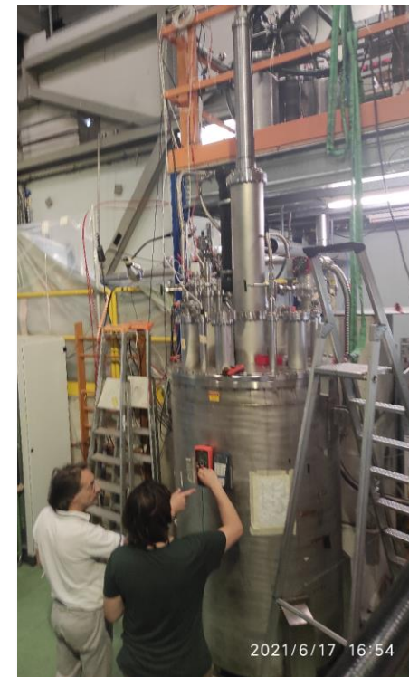
300 kV feedthrough test setup
