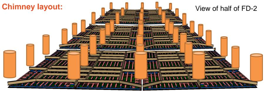
The position of the signal feedthroughs have been defined to avoid interference with the cryostat structure
