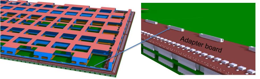
6 CRPs attached to a single Superstructure => 12 chimneys involved and 600 cables
