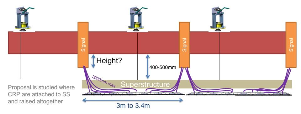
Signal cables are routed on the super-structure for each CRP, and have to be connected manually to chimneys.
