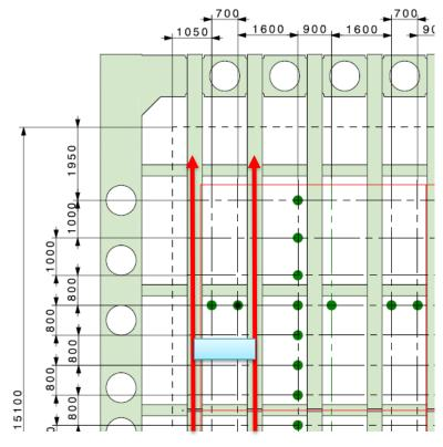
The crane rolls on the rails along the two I-beams, the pitch is 1.6 m
