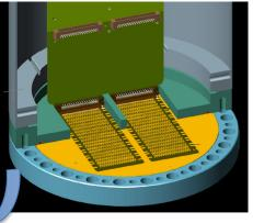
FE cards plugged on the cold flange at the bottom of the chimney
