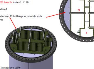
First design fitting 50 boards within defined diameter
