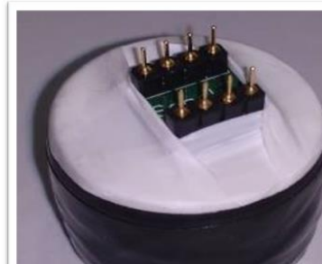
Lanthanum bromide 2x2 cm + Array 2x2 SiPM 3x3 mm
