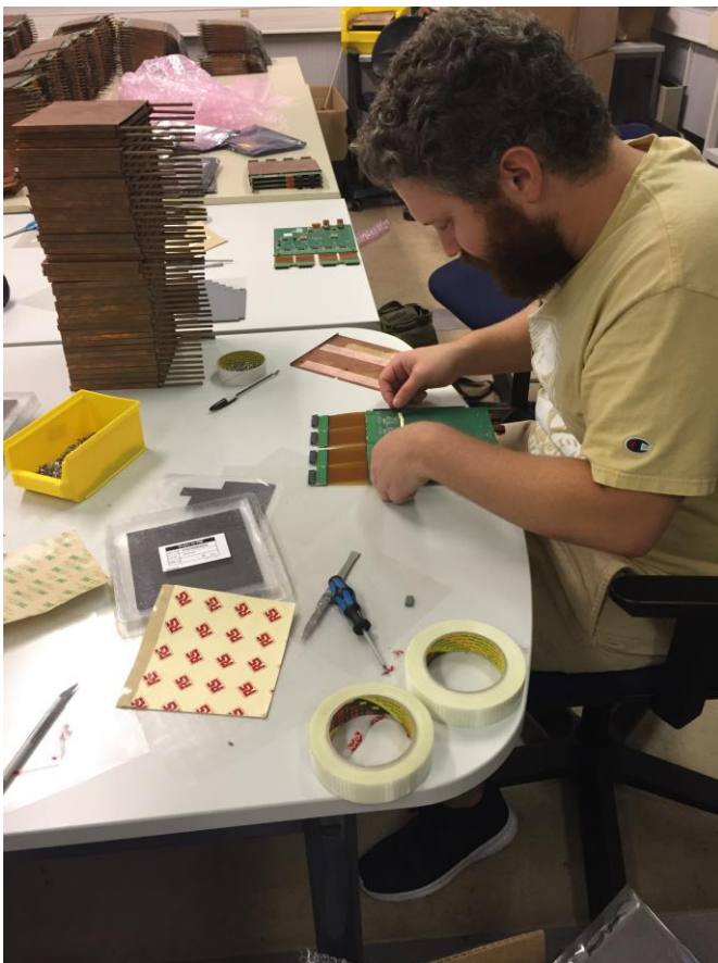
Thermal Pads on GBTx, SAMPAs, VTTx & VTRx, then seal w/ copper jacket
