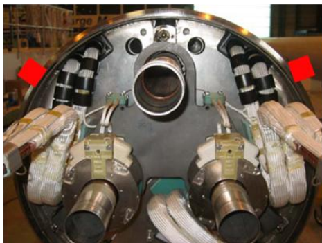
Figure 6: Position of material samples to be placed outside of the interconnects (red boxes).
