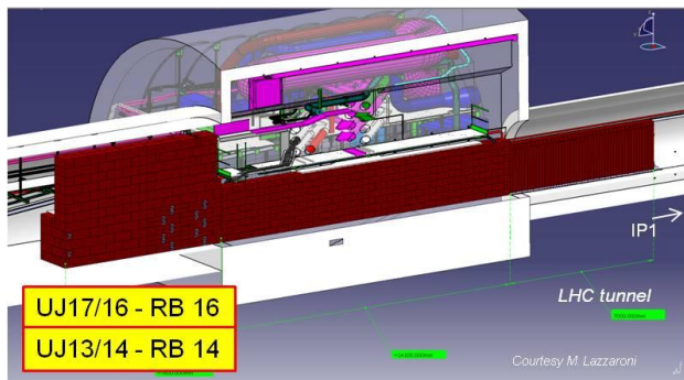
Figure 1c: New shielding implementation in UJs and RBs around Point 1.
