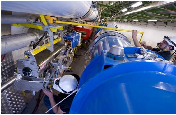
Figure 4: The transfer line collimators are located at the end of the lines where the transfer line is close to the LHC superconducting magnets. Showers created by the collimators are seen by the LHC beam loss monitors on the superconducting magnets.
