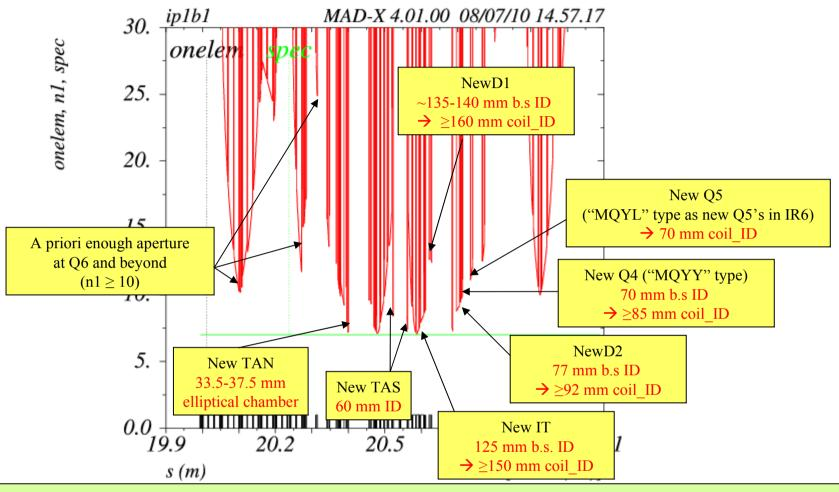
The above requirements are also compatible with a 15/15 cm  $\beta$ \*round optics and could be relaxed by ~10% (but for the TAS) with Nb3Sn triplet.
