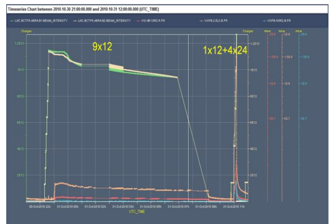
Fig. 1: Pressures and total intensity for the first two fills with 50 ns spacing. The gap in the data between 01:00 and 03:00 was due to an acquisition/logging problem related to the change from summer to winter time.
