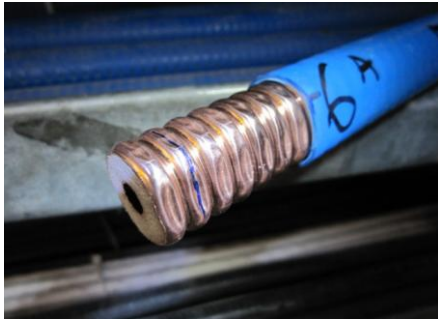
Figure 4: Damaged pick-up cable.
