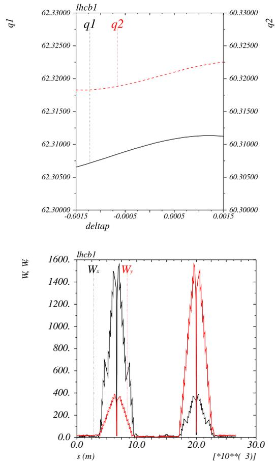
Figure 4: Chromatic variation of the betatron tunes (top) and chromatic Montague functions along the machine starting from IP7 (bottom) for the alternated flat collision optics shown in Fig. 3.
