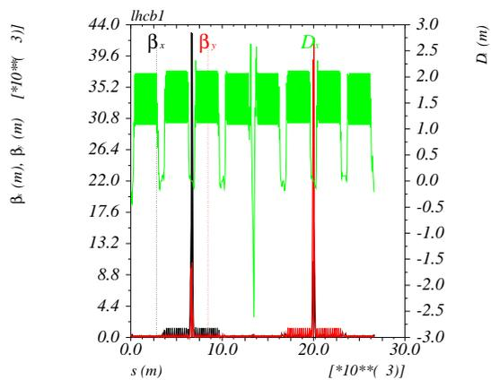
Figure 3: *Alternated flat collision optics for the HL-LHC with  $\beta_{x,y}^* = 7.5/30$  cm at IP1 and  $\beta_{x,y}^* = 30/7.5$  cm at IP5. Starting from a pre-squeezed optics with  $\beta_{x,y}^* = 60$  cm,  $\beta$ -beating waves are induced in the sectors 81, 12, 45 and 56 with peak values increased by a factor of 2 or 8 with respect to the regular FODO optics.*
