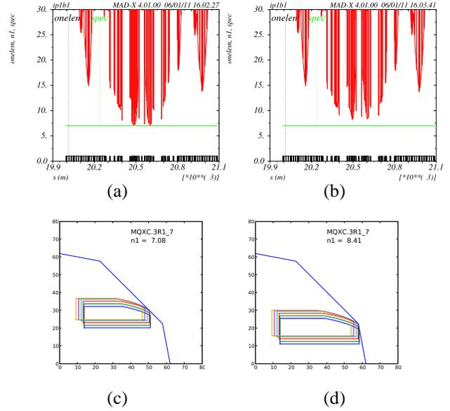
Figure 8: Aperture plots of the low- $\beta$  insertions (top) and extension of the secondary halo inside the octagonal beam-screen of Q3 (bottom) assuming the optics and the transverse emittance given in Tab. 4, and considering the initial and final crossing angle specified at the beginning (left) and end (right) of the physics coast.
