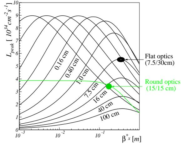
Figure 2: Peak Luminosity as a function of  $\beta^*$  in the crossing plane for different values of  $\beta^*$  in the other plane (full crossing angle of  $10\sigma$ , so-called “ultimate” beam parameters with 25 ns bunch spacing,  $1.7E11$  p/bunch,  $\gamma\epsilon = 3.75\text{ }\mu\text{m}$ ,  $\sigma_z = 7.5\text{ cm}$ ). The green line stands for the case of round collision optics ( $\beta_x^* = \beta_y^*$ ).
