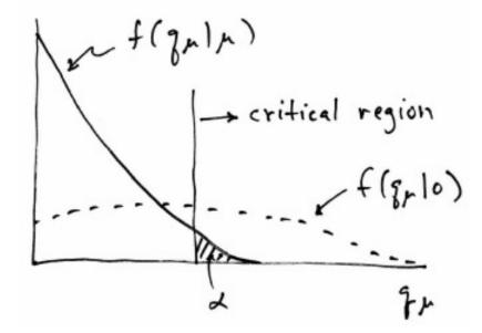
That is, the power (probability to reject  $\mu$  if  $\mu = 0$ ) is substantially higher than  $\alpha$ . Use this power as a measure of the sensitivity.
