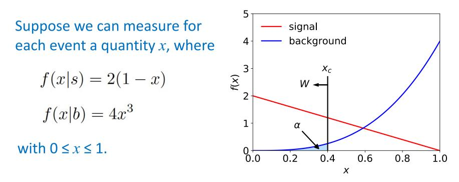
For each event in a mixture of signal (s) and background (b) test
