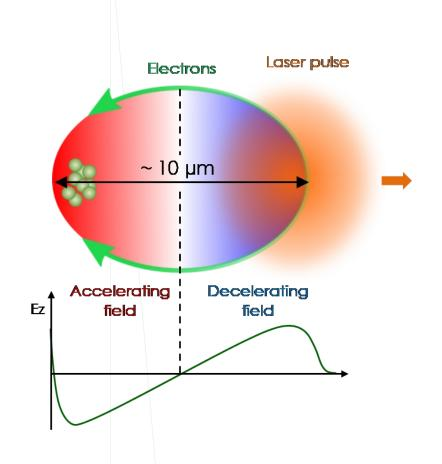
Extracting most of the laser energy and reaching high-energy requires to sustain a high amplitude electric field over a long distance
