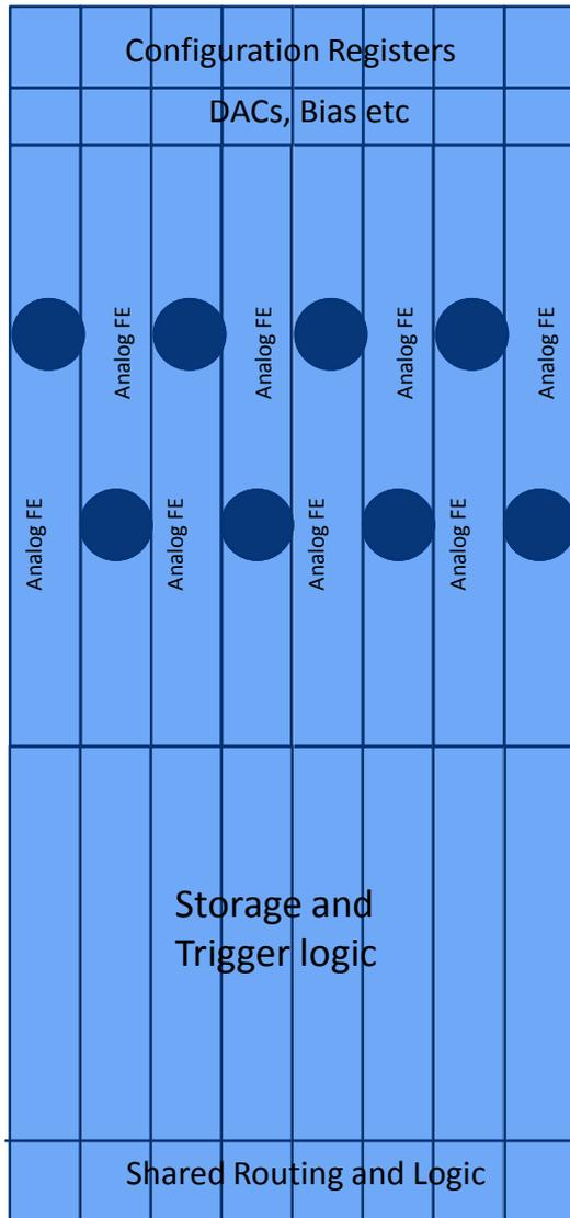
Single Pixel size:  $100 \times \sim 1400 \mu\text{m}^2$
